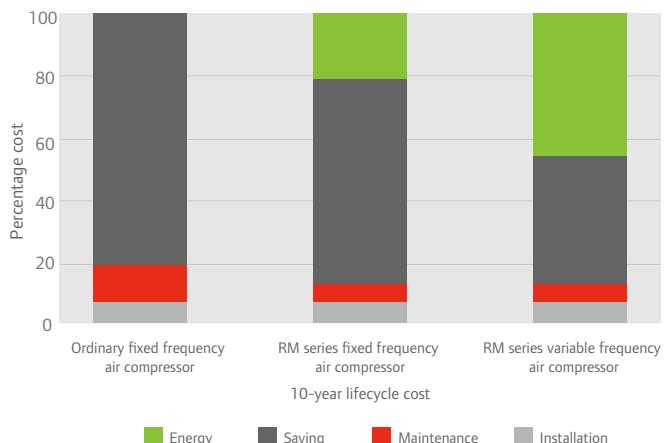
Running at a load of 79%; Running for 4000 hours per year; 0.05\$/kWh
